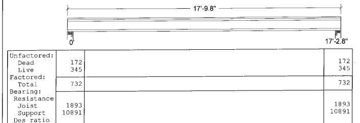
Kzcp sup | 1.15 | Bearing for wall supports is perpendicular-to-grain bearing on top plate. No stud design included.
