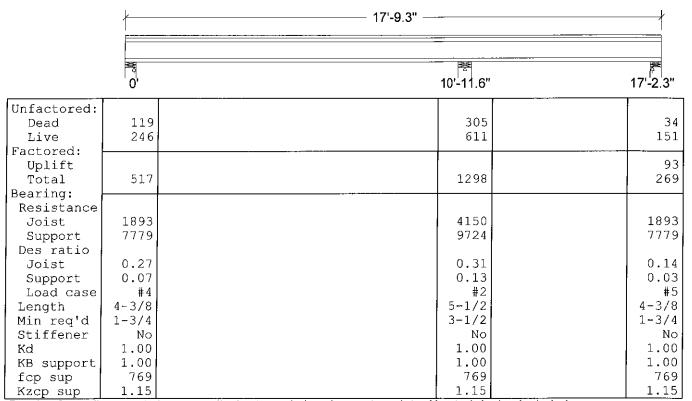
Bearing for wall supports is perpendicular-to-grain bearing on top plate. No stud design included.
